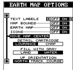
The unit returns to the mapping screen with the message "Set Map Center" flashing at the bottom of the screen. Use the arrow keys to move the present position indicator to the desired location on the screen, then press the EXIT key. This locks the present position indicator in this location.
