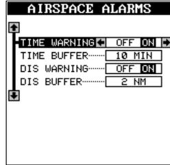
To adjust an alarm, or turn it on or off, move the black box to the desired label, then press the right or left arrow keys. When you have everything on this page set as desired, press the EXIT key to erase this menu and return to the ALARMS menu.
