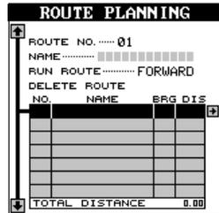
You can place a waypoint using the waypoint list or from locations on the map, or both. For the first waypoint, we'll use the "Insert From WPTS" method. With the black box on this menu, press the right arrow key. A screen similar to the one below appears.
