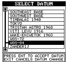
The WGS-84 label is highlighted. To change it, simply press the up or down arrow keys until the desired datum is highlighted, then press the ENT key. This selects the datum and erases the datum menu. The AirMap 300 is now using the datum you selected.
