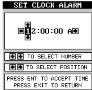
To turn the alarm on, press the MENU key, then select the “CLK ALM” menu. Press the right arrow key. The alarm is now activated.
