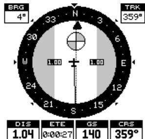
The digital boxes at the bottom of the screen show (from left to right) your distance to go to the destination (DIS), estimated time en route (ETE), ground speed (GS), and course (CRS). Course (CRS) is the bearing from your starting location to your destination. (Remember,
