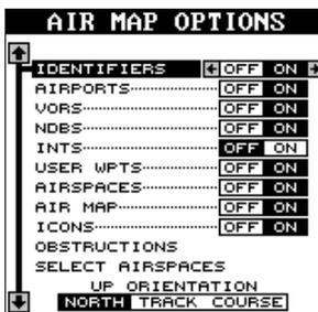
Use the up and down arrow keys to move the box to the desired symbol, then press the right arrow key to turn it on or the left arrow key to turn it off.
