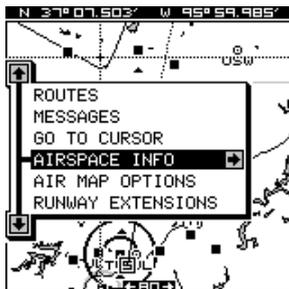
This is the information for the airspace that the cursor is resting on. To view information about another airspace, simply move the cursor to that airspace and repeat these steps. To erase this screen, simply press the EXIT key.
