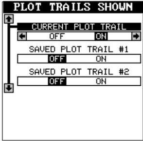
Use the up or down arrow keys to select the desired plot trail, then press the left or right arrow key. Press the EXIT key to return to the Plotter Options menu.
