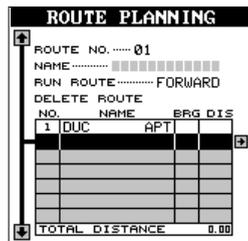
Continue selecting waypoints until the route is complete. As you add waypoints to the list, the bearing and distance from each waypoint to the one previous is shown to the right of the waypoint's name. In this example, the second waypoint in the list is 104 degrees and 30.75 miles from the first waypoint in the list.
