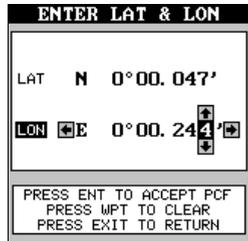
After you’ve entered the latitude/longitude correction, press the ENT key to accept it. The AirMap 300 returns to the navigation or mapping screens with the correction factor applied.
