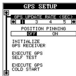
If you wish to turn the position pinning feature on, press the MENU key, then highlight the “GPS Setup” label and press the right arrow key. Now highlight the “Position Pinning” label. Finally, press the right arrow key.
