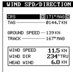
our course is 171° magnetic. This gives us a wind speed of 11.5 knots on a bearing of 234° true, for a 6 knot headwind.
