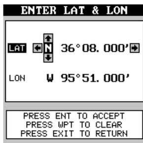
Keep pressing the arrow keys until the latitude and longitude are set to your local position. (Note: This position does not have to be very accurate. If you can get it within one degree of your actual position, that will be fine.) When it's set, press the ENT key. The AirMap 300 accepts your entry and returns to the GPS setup menu.
