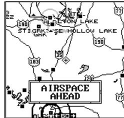
When an alarm is triggered, the AirMap 300 flashes a message on the screen as shown at right. To view the airspace information, switch to the “Messages” mode.
