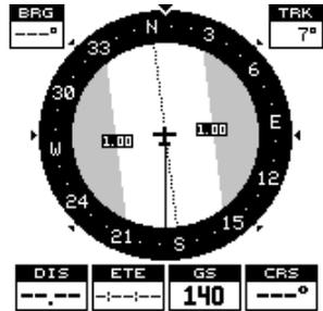
Your speed over ground or Ground Speed is shown at the bottom of this screen. In this example, the ground speed is 140 knots. The screen looks like this when you're not navigating to a waypoint. (See page 58 for information on waypoint navigation.) If you navigate to a waypoint, the screen looks like the one below.
