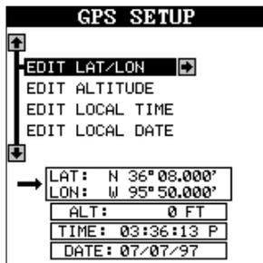
Once the AirMap 300 finds and locks on to three satellites, it stops flashing the numbers on the display. (Note: Altitude will still flash until the unit locks on to the fourth satellite. It takes four satellites to determine altitude.)
