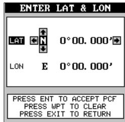
Now enter the correction for your location. Remember, this is the difference between the location shown on the present position display and the position shown on the chart. In this example, we entered 0 degrees, 0.047 minutes north latitude and 0 degrees, 0.244 minutes east longitude. That is the difference between the present position shown by the AirMap 300 and the one on our chart.
