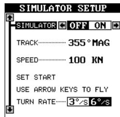
If you simply press the right arrow key, turning the simulator on, the AirMap 300 will start from your present position and "fly" a track of 355° at 100 knots.
