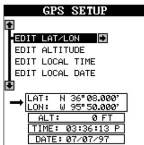
To change the position, highlight the “EDIT LAT/LON” label, then press the right arrow key. A screen similar to the one at right appears. With the “INPUT FROM MAP” label highlighted, press the right arrow key. The screen below appears.
