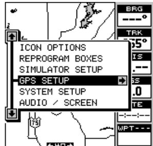
Using the down arrow key, highlight the “Initialize GPS Receiver” menu, then press the right arrow key. The screen shown below appears next.
