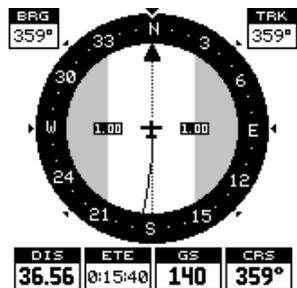
The numbers on either side of the center arrow show the cross track error range. In other words, (using the screen at right as an example) if the arrow crosses the dark band on either side, you are one mile to the left or right of the desired course.
