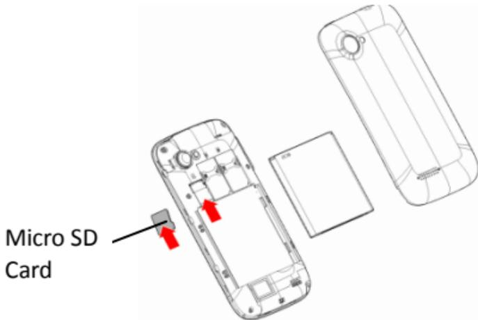
3. Finally insert the battery and the rear cover of the mobile phone.
