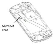
Finally insert the battery and the rear cover of the mobile phone.
