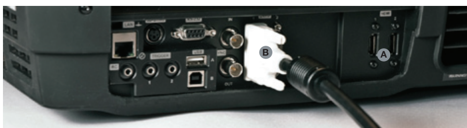
Figure 5-5. Connecting a computer source
