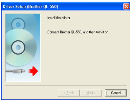
**8** When the Driver Setup dialog box instructs you to connect the QL-500/550, plug the connector on the USB cable into the USB port on the back of the QL-500/550.
