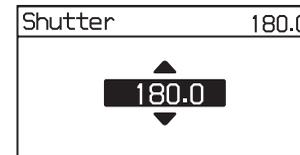
You do not need to press the MENU SEL/ENTER dial to set a value. The shutter value changes are reflected on the camera as the MENU SEL/ENTER dial is turned. Pressing the BACK button cancels the shutter setting, and restores the previous value.
