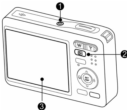
**2** Press the **POWER** button (❶) again to turn the power off.
