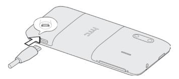
Plug the AC adapter into an electrical outlet. Fully charging a battery may take up to three hours.
