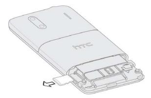
5. Replace the microSD card and the battery compartment cover.
