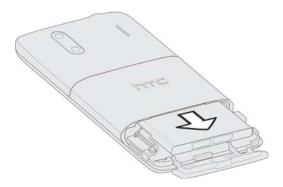
• Insert the battery back into the slot, contacts side first, and then close the battery compartment door to lock the battery in place.
