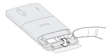
Pull out the battery, and then remove the film that covers it.
