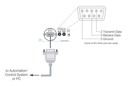
Figure 3-11. RS-232 Control System Connection
