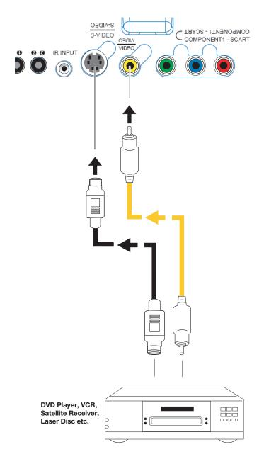
**Composite/S-Video Connections:** Connect your Composite and S-Video sources to the LS-7 as shown in Figure 3-10.
