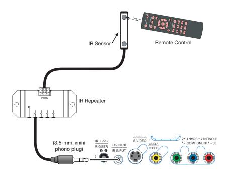
Figure 3-13. External IR Receiver Connection
